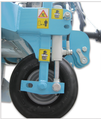
Hydraulically adjustable front wheel controls cultivating depth
