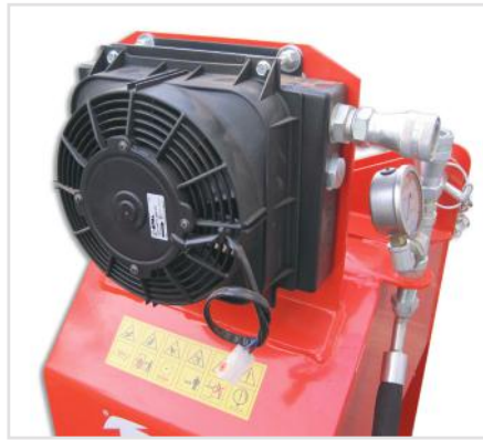
Return oil cooler with fan
